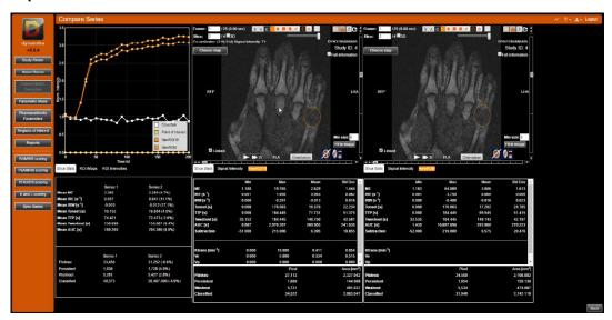
The *Compare Series* screen offers comprehensive slice statistics alongside each series. It also offers signal-time curve visualisation for dynamic series in the top left pane.
